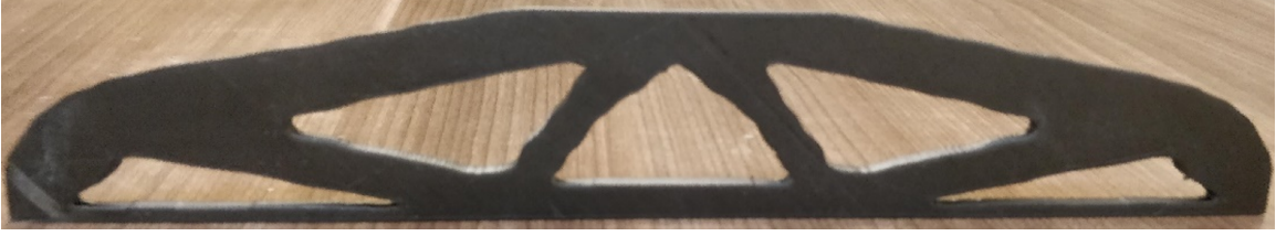
Figure 5.12: 3D printed beam from an STL file generated by processing a smooth boundary image.
