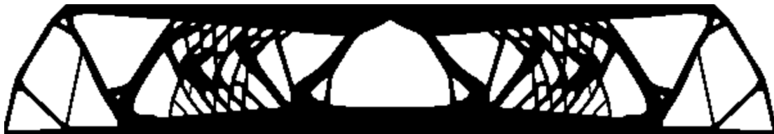
Figure 5.7: Criss-cross topology pattern shown by an optimized MBB topology obtained with the reciprocal interpolation technique, 300-by-100 mesh, \beta = 0.25 , \zeta = 10^9 for a 90 degree transversely isotropic material
